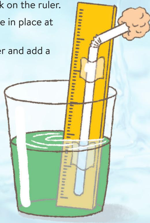
6. Measure how high the water rises in the straw, and note it on a piece of paper. Every day, check your barometer and see if the level has changed.
